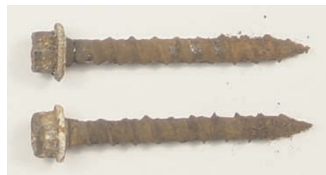
ACQ treated lumber – heavy rust, loss of threads and holding power
