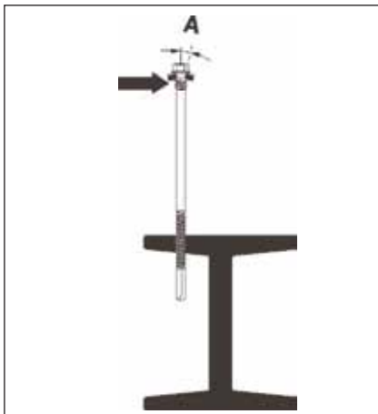
ECCS repetitive bending tests on SFS intec composite panel fasteners
