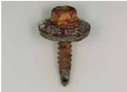
Corrosion of nitrided stainless
