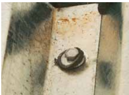
Poor washer design
